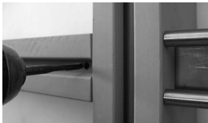
M5-Gewinde schneiden Filetage M5 Cut M5 thread
